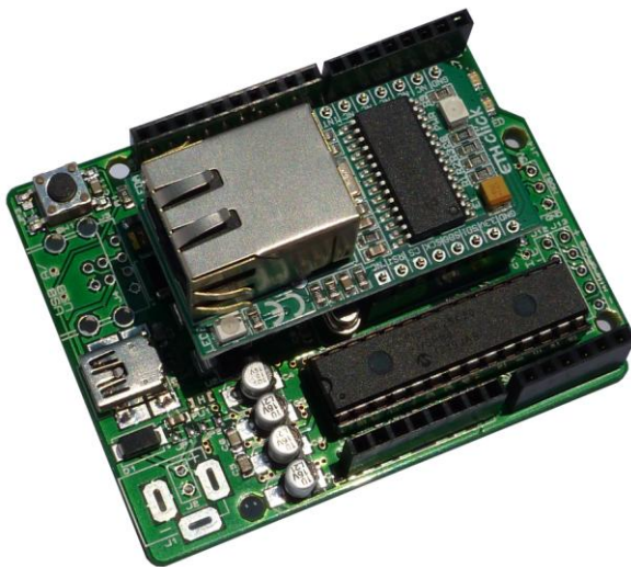
“ETH click” Ethernet board connected
