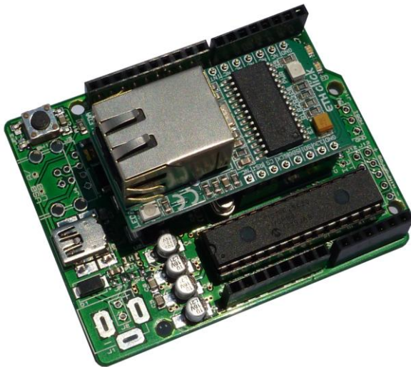
“ETH click” Ethernet board connected
